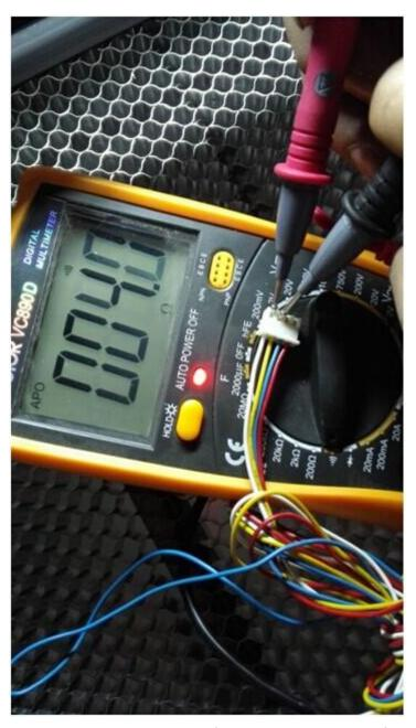
2 connected two groups cables of stepper motor with the left driver board. In left drive board has two thick cables like attached 1, please connected two groups cables with A+ A- and B+ B- in left
